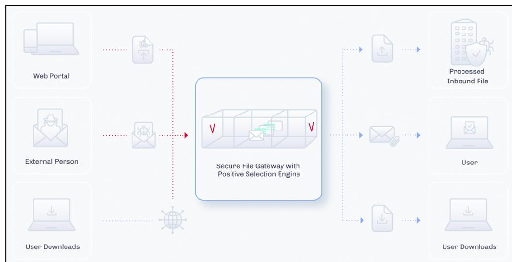
Data flows between Positive Selection Engine, Votiro's Secure File Gateway for Web Applications, Secure File Gateway for Email and Secure File Gateway for Web Downloads. Communication consists of multiple bi-directional messages that include queuing, tracking, file transfers and reports.
